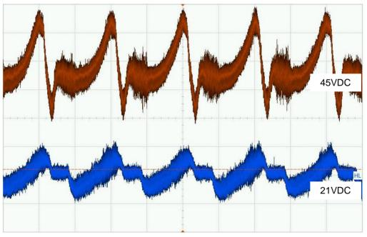
Figure 10: 100Hz Output current ripple, full load & half load 230VAC (10mA/div)
