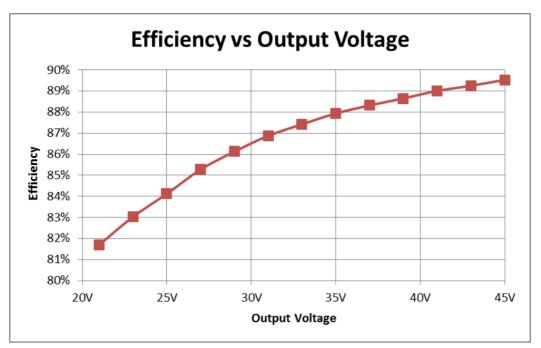
Figure 3: Efficiency @ 230VAC over output voltage range
