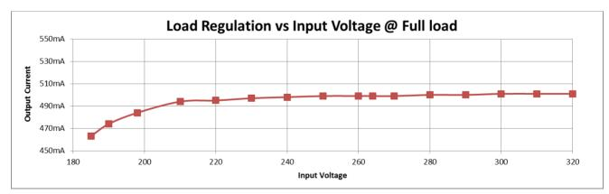
Figure 5: Output regulation over a wide mains input range (full load 45V out)
