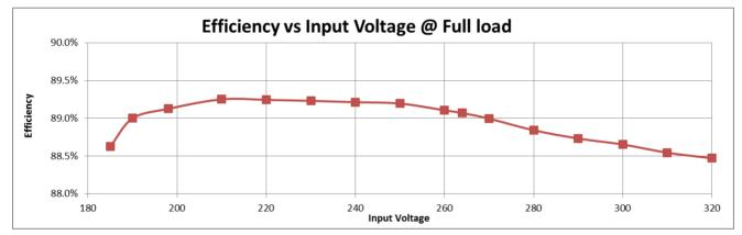
Figure 4: Efficiency over a wide mains input range (full load 45V out)
