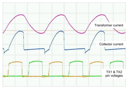
Figure 9: Base drive waveforms, TX1, TX2, transistor current, total current
