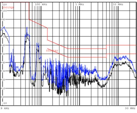
Figure 11: 22W driver conducted emissions
