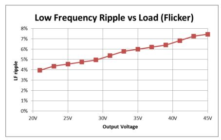
Figure 6: Low Frequency ripple (Flicker) @ 230V over output voltage
