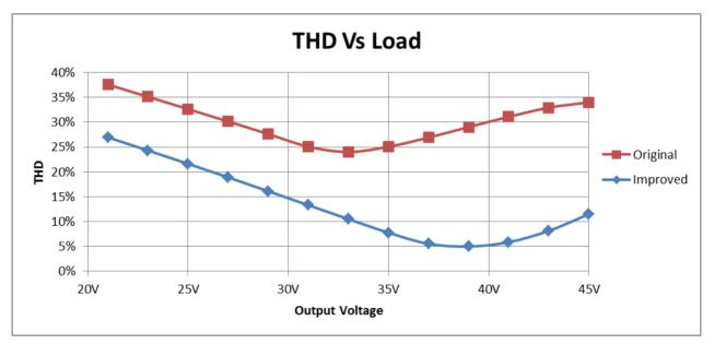
Figure 13: THD @ 230V over output voltage (original vs Improved)
