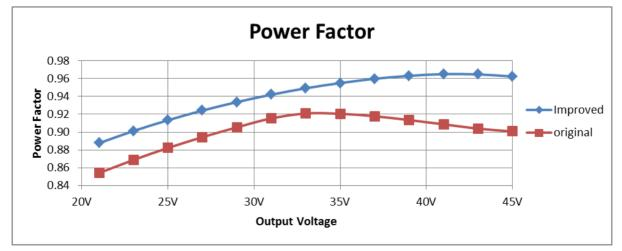
Figure 14: Power Factor @ 230V over output voltage (original vs Improved)
