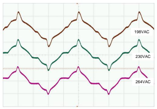
Figure 7: 50Hz Input current 22W @ 198, 230, 264VAC
