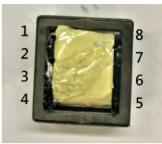
Note that Pin4 is connected to the "hot" noisy end of the winding. This keeps the noisy end of the winding on the inside of the bobbin and the quieter end on the outside to act as a screen. If the converter is being affected by noise, the core can be connected to a quiet point.
