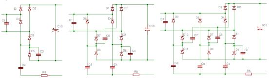
Figure 5: single, double and triple boost stages
