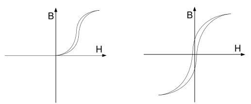
Figure 2: Flyback compared to LLC transformer Flux Density swing
