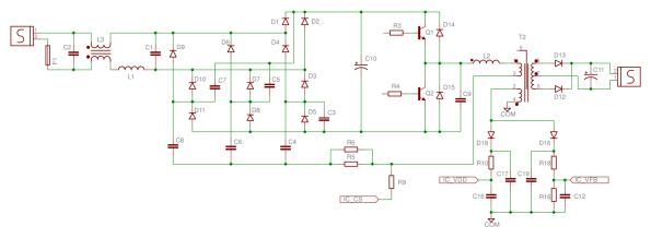
Figure 1: RediSem driver key component reference schematic
