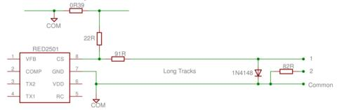
Figure 1: Current selection on the IC's CS pin
