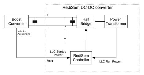
Figure 4: Complete system with Aux connected
