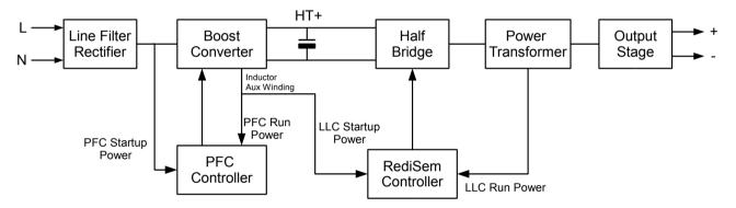
Figure 1: APFC Powering Configuration
