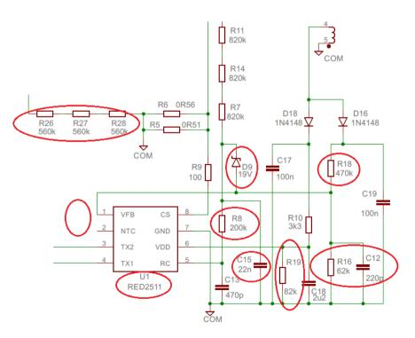
Figure 3: Changes required to turn the IC off at high voltages
