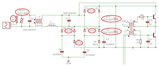
Figure 2: Modifications for 400VAC operation
