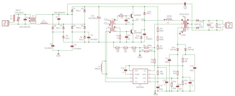
Figure 1: Standard 42W schematic for 320VAC operation
