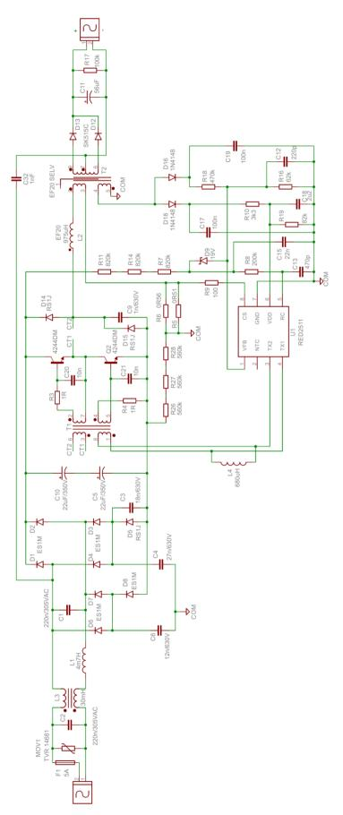
Figure 4: Full schematic to support 460VAC survival and 6kV surge
