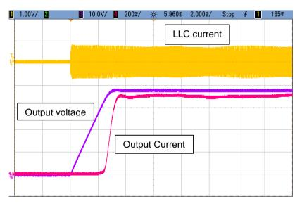
Figure 1: Normal startup with an LED load
