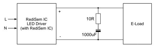
Figure 3: Startup helping circuit
