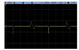
Figure 11: output voltage with load steps 0-10%
