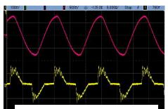
Figure 13: Primary current and CS pin waveforms
