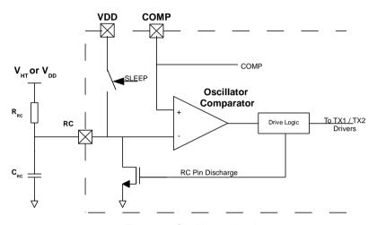
Figure 8: Oscillator circuit
