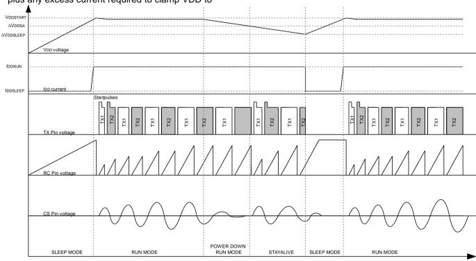
Figure 4: IC Start-up waveforms
