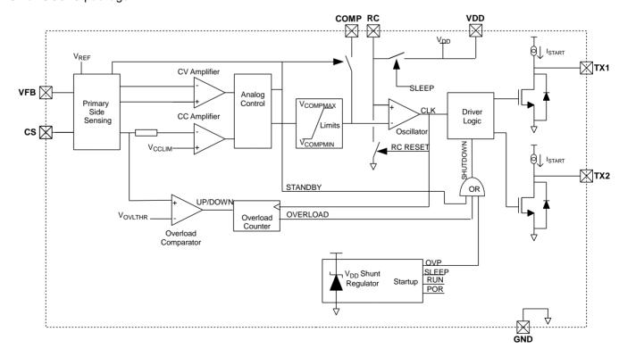
Figure 1: Block diagram
