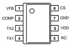
Figure 2: SO8 pin connections (top view)
