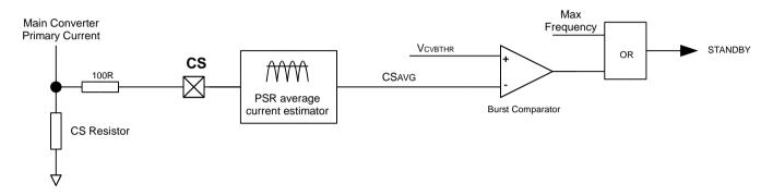
Figure 9: standby entry circuit
