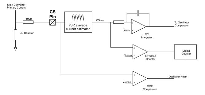
Figure 7: RED1401 Current protection and control circuits
