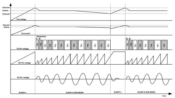
Figure 4: RED2101 Startup waveforms
