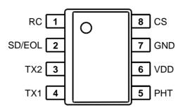
Figure 2: SO-8N pin connections (top view)
