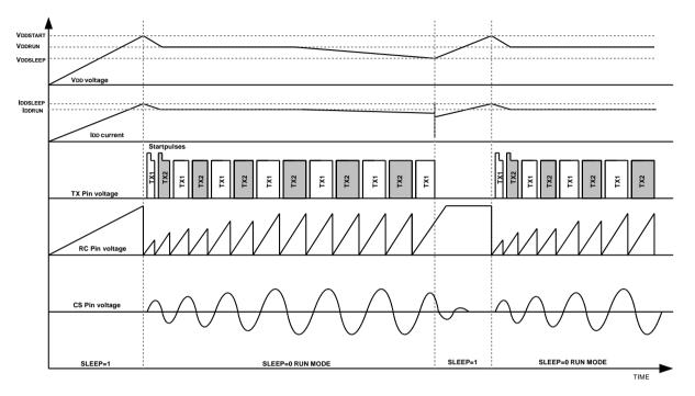
Figure 5: RED2201 Startup waveforms
