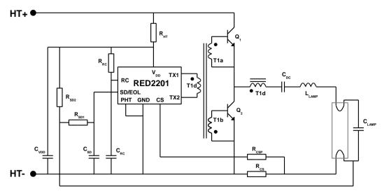
Figure 3: RED2201 Application diagram
