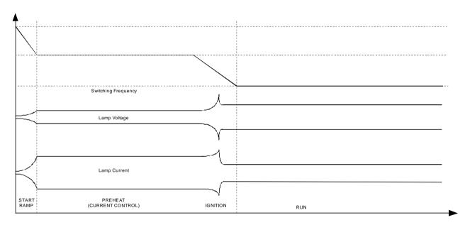
Figure 6: Ballast operating modes with RED2201
