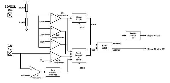
Figure 7: Fault protection circuit inside RED2201
