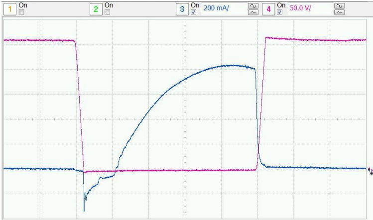
Collector current and voltage
