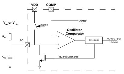
Figure 8: Oscillator circuit
