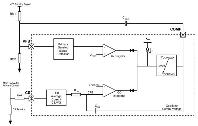
Figure 6: Error Amplifier Circuits
