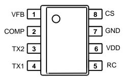
Figure 2: SO8 pin connections (top view)
