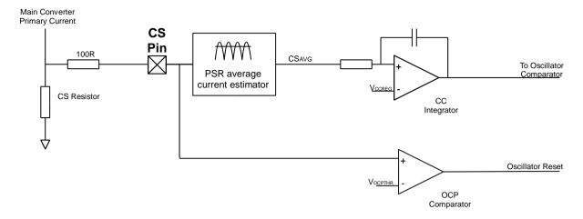
Figure 7: RED2501 Current protection and control circuits
