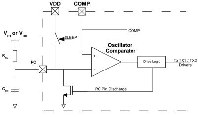
Figure 8: Oscillator circuit
