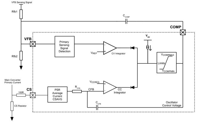
Figure 6: Error Amplifier Circuits
