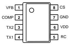
Figure 2: SO8 pin connections (top view)
