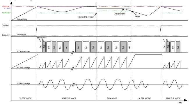
Figure 4: IC Start-up waveforms
