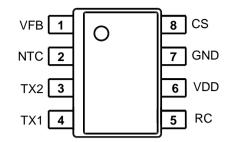
Figure 2: SO8 pin connections (top view)
