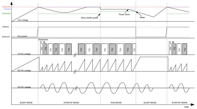
Figure 4: IC Start-up waveforms
