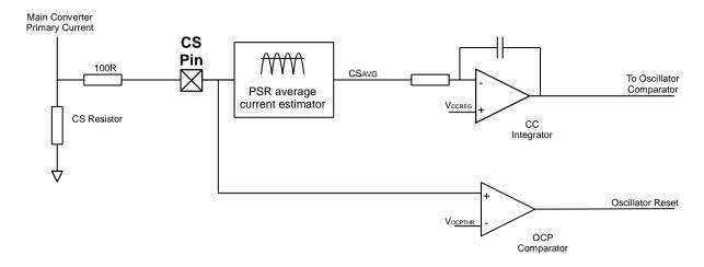
Figure 7: RED2521 Current protection and control circuits
