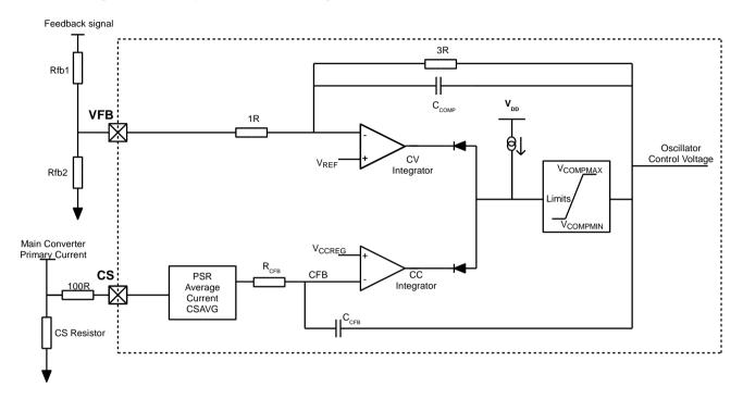
Figure 6: Error Amplifier Circuits
