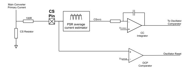
Figure 7: RED2541 Current protection and control circuits
