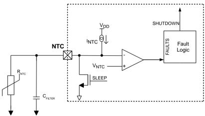
Figure 9: RED2541 NTC pin circuit
