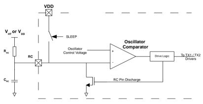
Figure 8: Oscillator circuit
