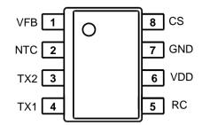
Figure 2: SO8 pin connections (top view)
