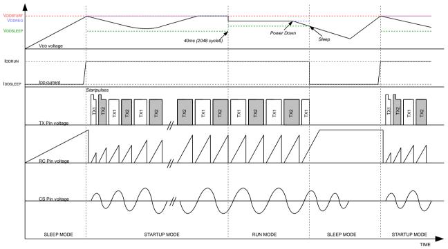
Figure 4: IC Start-up waveforms
