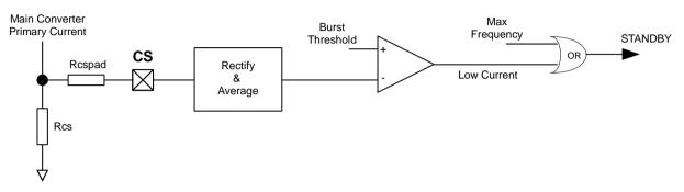
Figure 6: Standby Entry Circuit
