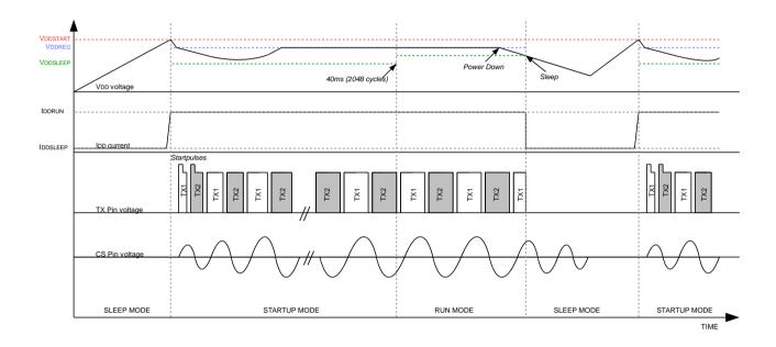
Figure 4: IC Start-up waveforms
