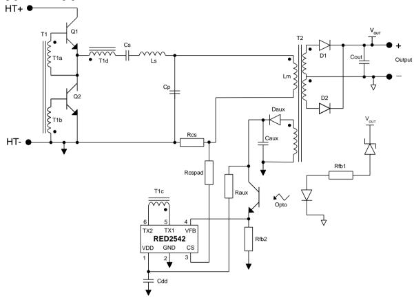
Figure 3: Typical Application Schematic: LLC converter with RED2542 CV controller
