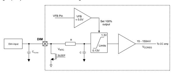
Figure 10: RED2821 DIM pin circuit
