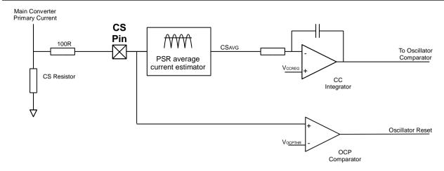
Figure 8: RED2821 Current protection and control circuits
