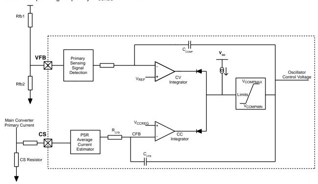
Figure 7: Error Amplifier Circuits
