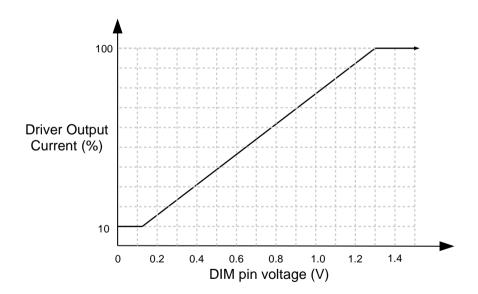
Figure 11: DIM pin voltage vs output current
