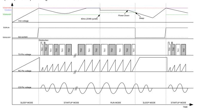
Figure 5: IC Start-up waveforms
