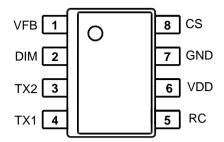
Figure 2: SO8 pin connections (top view)
