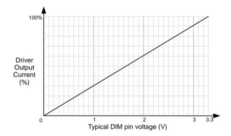
Figure 9: DIM pin voltage vs output current
