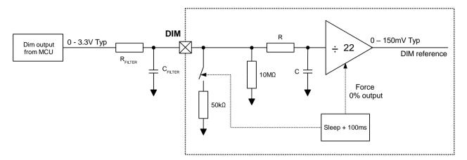
Figure 8: RED2822 DIM pin circuit
