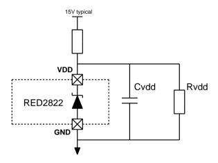
Figure 4: VDD & GND connections
