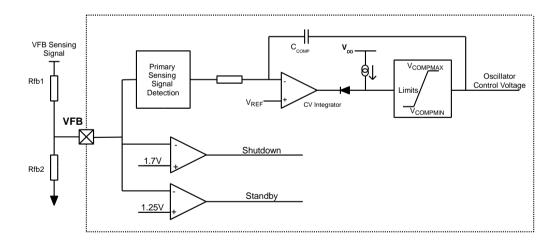
Figure 6: Voltage Error Amplifier Circuit
