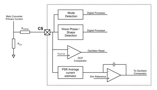
Figure 7: CS Pin connection
