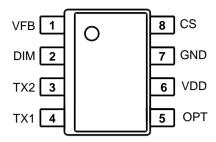
Figure 2: SO8 pin connections (top view)
