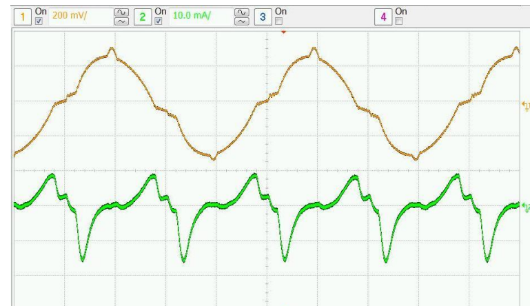
Input current and output flicker current
