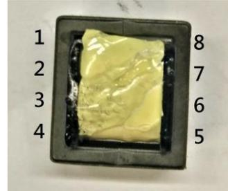
Note that Pin4 is connected to the "hot" noisy end of the winding. This keeps the noisy end of the winding on the inside of the bobbin and the quieter end on the outside to act as a screen. If the converter is being affected by noise, the core can be connected to a quiet point.
