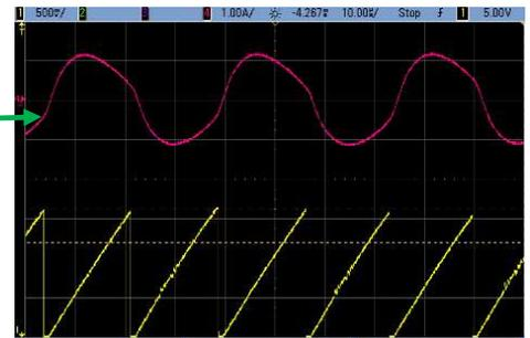
Figure 9: Primary current and RC pin on edge of capacitive mode switching (zoomed in)
