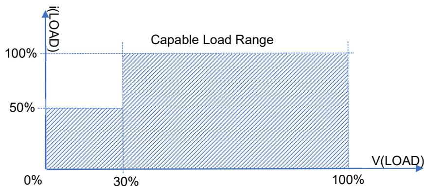
Figure 5: Static characteristics of allowed loads
