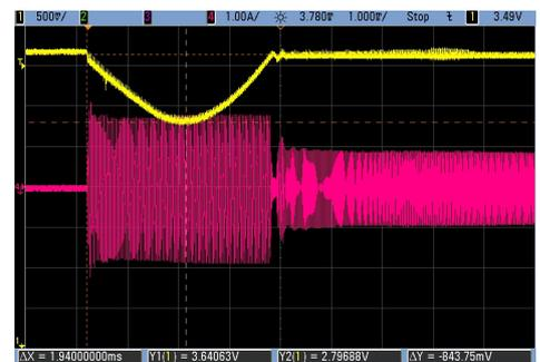
Figure 6: VDD, primary current (good startup)
