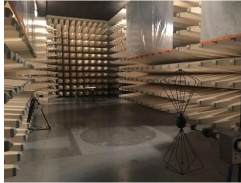
Radiated Test Setup
