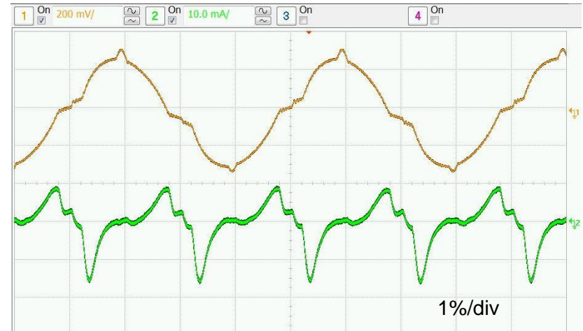
Input current and output flicker current
