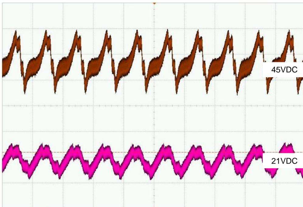
Figure 12: 100Hz Output current ripple, full load & half load 230VAC (20mA/div)
