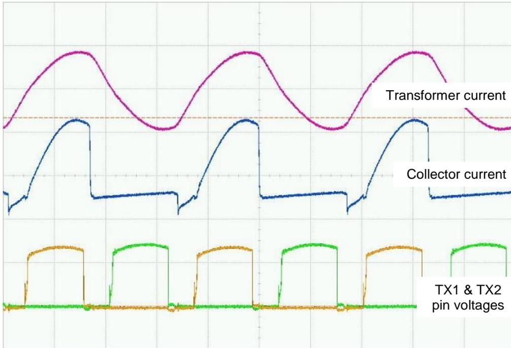
Figure 11: Base drive waveforms, TX1, TX2, transistor current, total current
