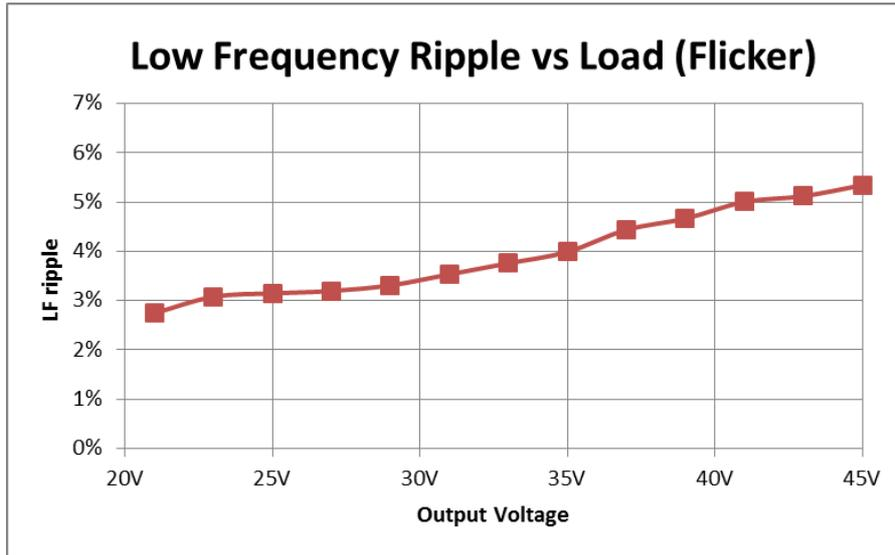
Figure 6: Low Frequency ripple (Flicker) @ 230V over output voltage
