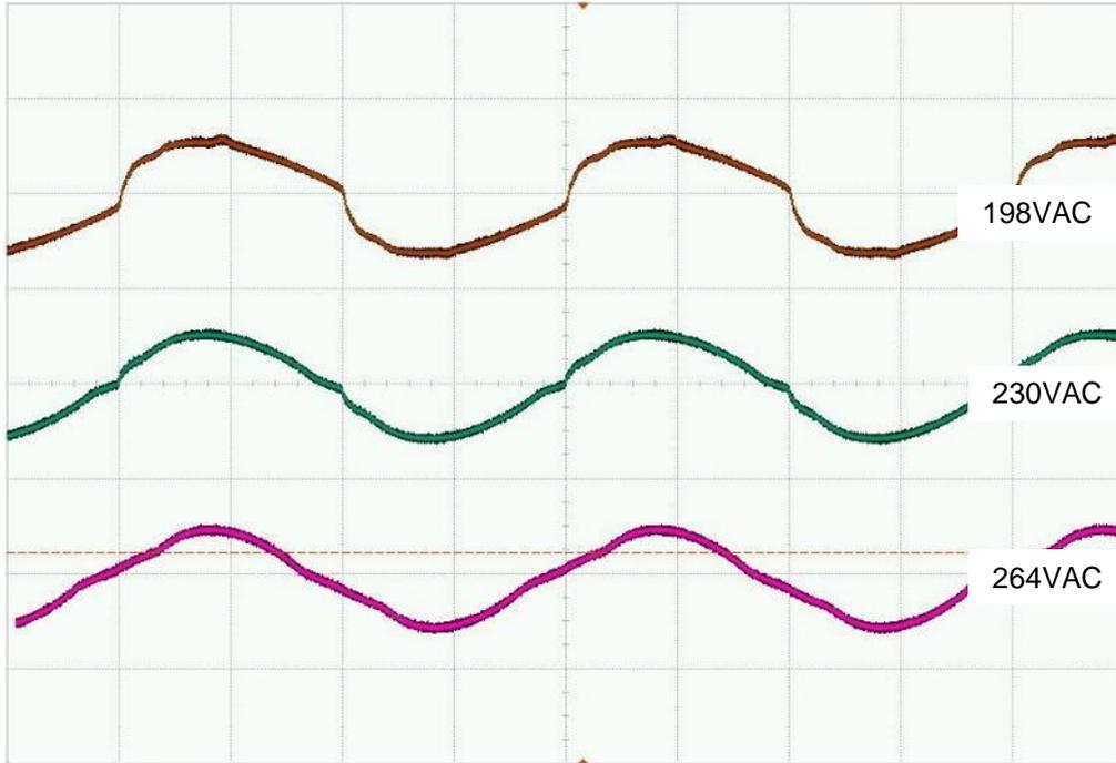
Figure 9: 50Hz Input current 40W @ 198, 230, 264VAC
