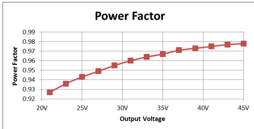
Figure 8: Power Factor @ 230V over output voltage
