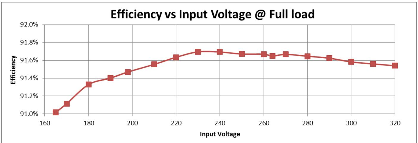
Figure 4: Efficiency over a wide mains input range (full load 45V out)
