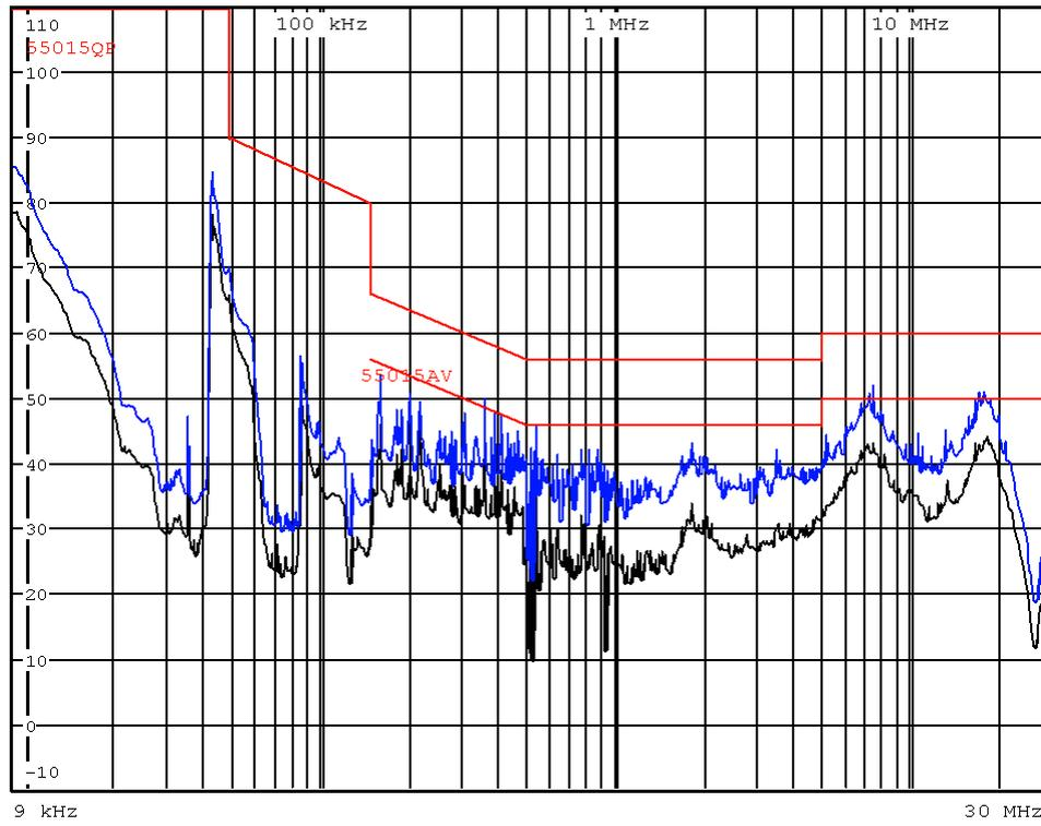
Figure 13: 40W driver conducted emissions
