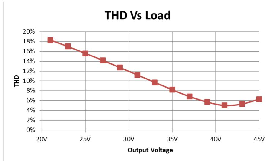
Figure 7: THD @ 230V over output voltage
