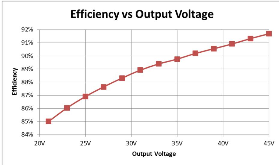
Figure 3: Efficiency @ 230VAC over output voltage range
