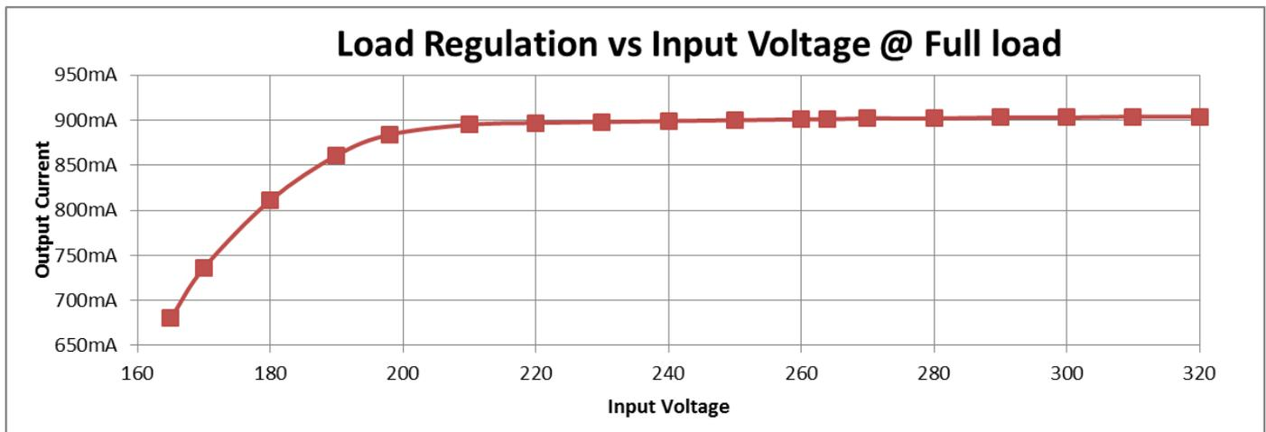
Figure 5: Output regulation over a wide mains input range (full load 45V out)
