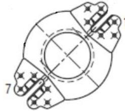
Note that Pin1 is connected to the “hot” noisy end of the winding. This keeps the noisy end of the winding on the inside of the bobbin and the quieter end on the outside to act as a screen. If the converter is being affected by noise, the core can be connected to a quiet point.
