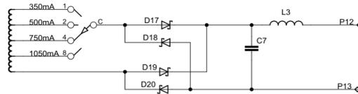
Figure 3: Switchable outputs
