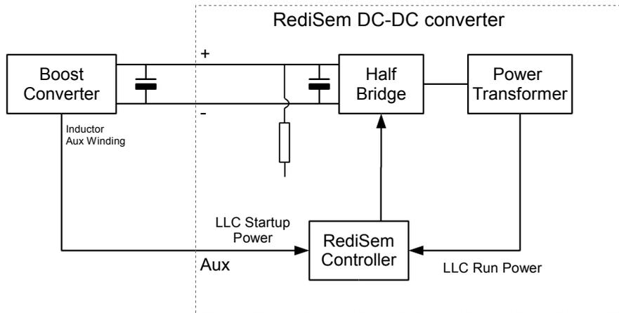
Figure 4: Complete system with Aux connected
