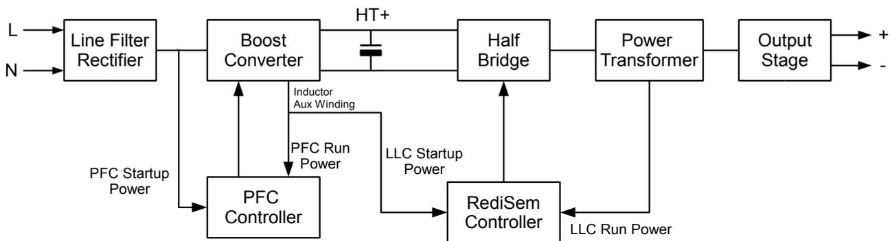
Figure 1: APFC Powering Configuration
