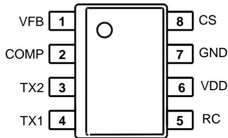
Figure 2: SO8 pin connections (top view)
