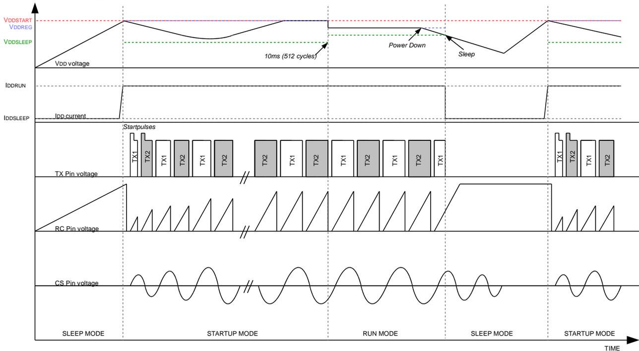
Figure 4: IC Start-up waveforms
