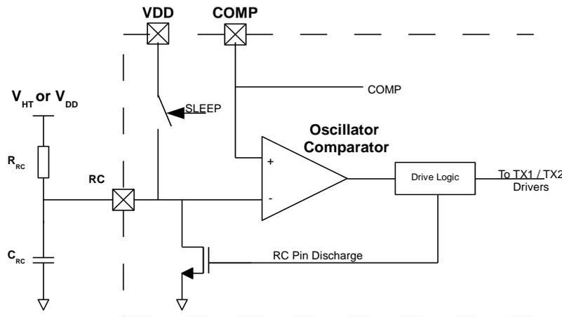
Figure 8: Oscillator circuit
