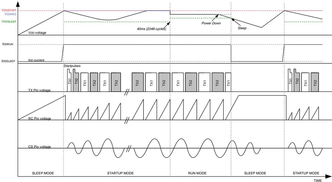
Figure 4: IC Start-up waveforms
