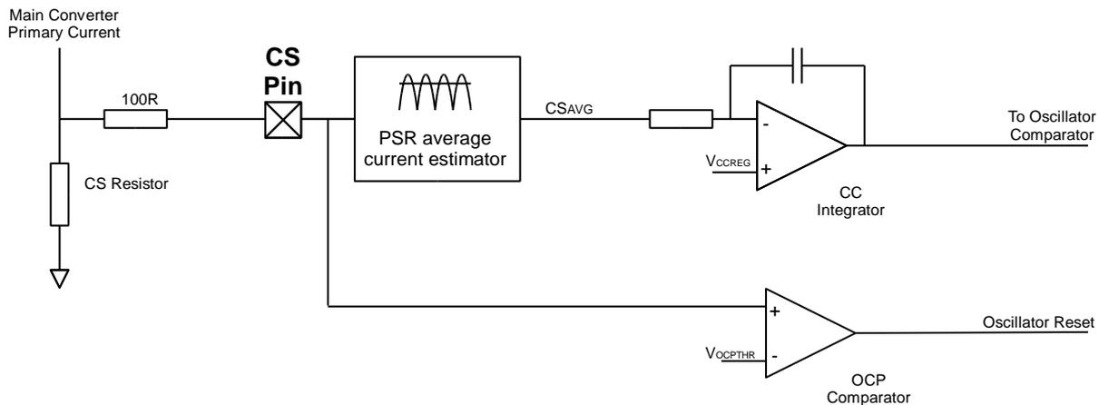
Figure 7: RED2521 Current protection and control circuits
