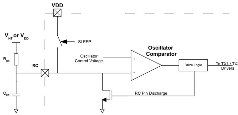
Figure 8: Oscillator circuit
