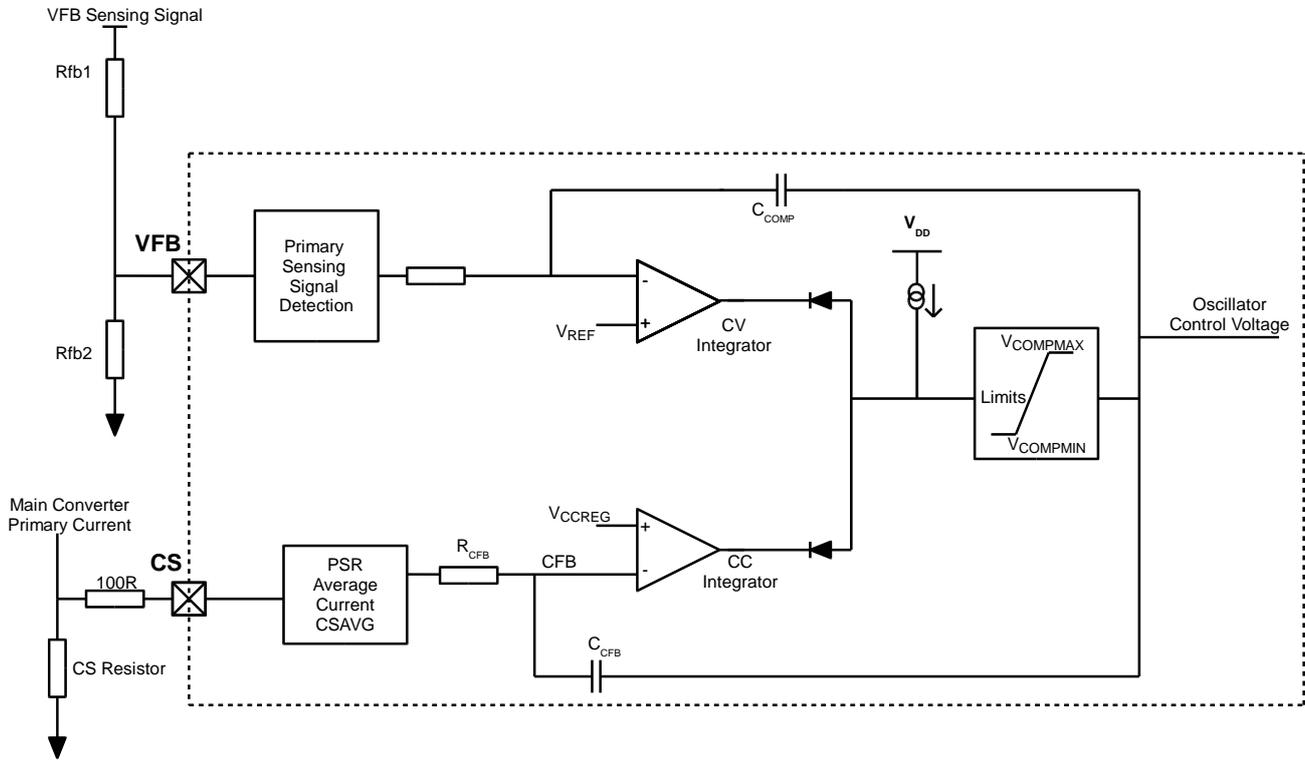
Figure 6: Error Amplifier Circuits
