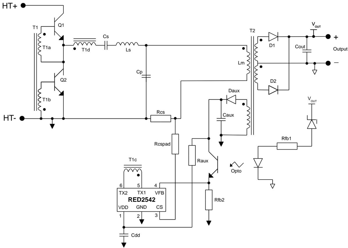
Figure 3: Typical Application Schematic: LLC converter with RED2542 CV controller
