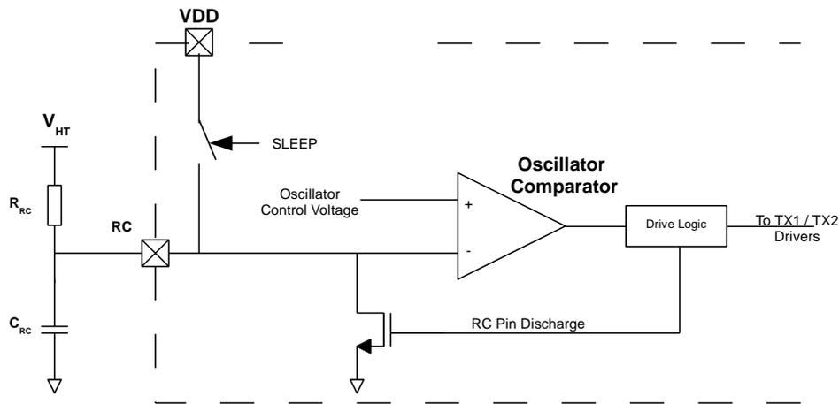
Figure 9: Oscillator circuit
