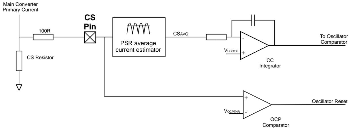
Figure 8: RED2821 Current protection and control circuits
