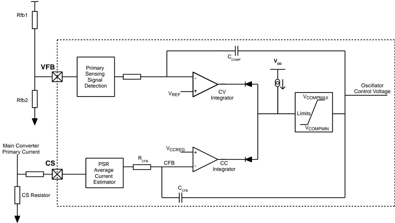
Figure 7: Error Amplifier Circuits
