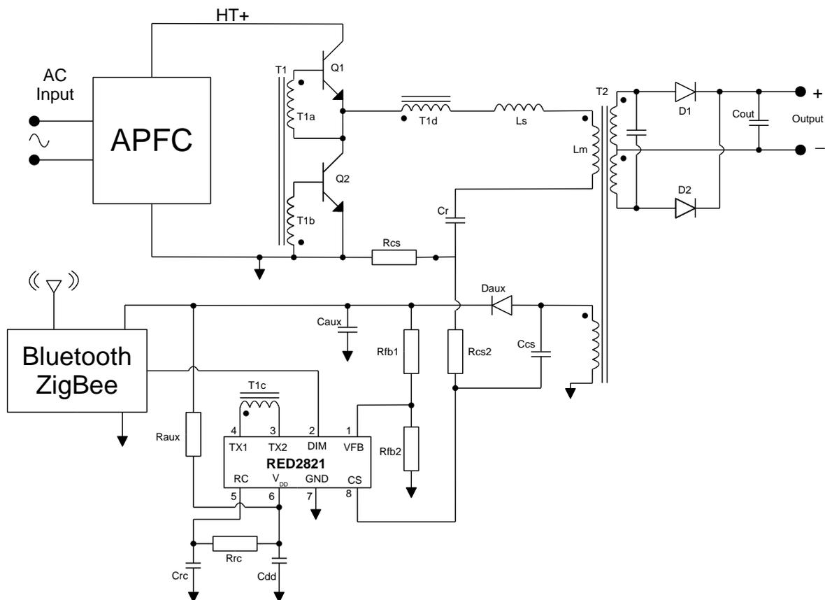
Figure 4: Application showing wireless primary side control
