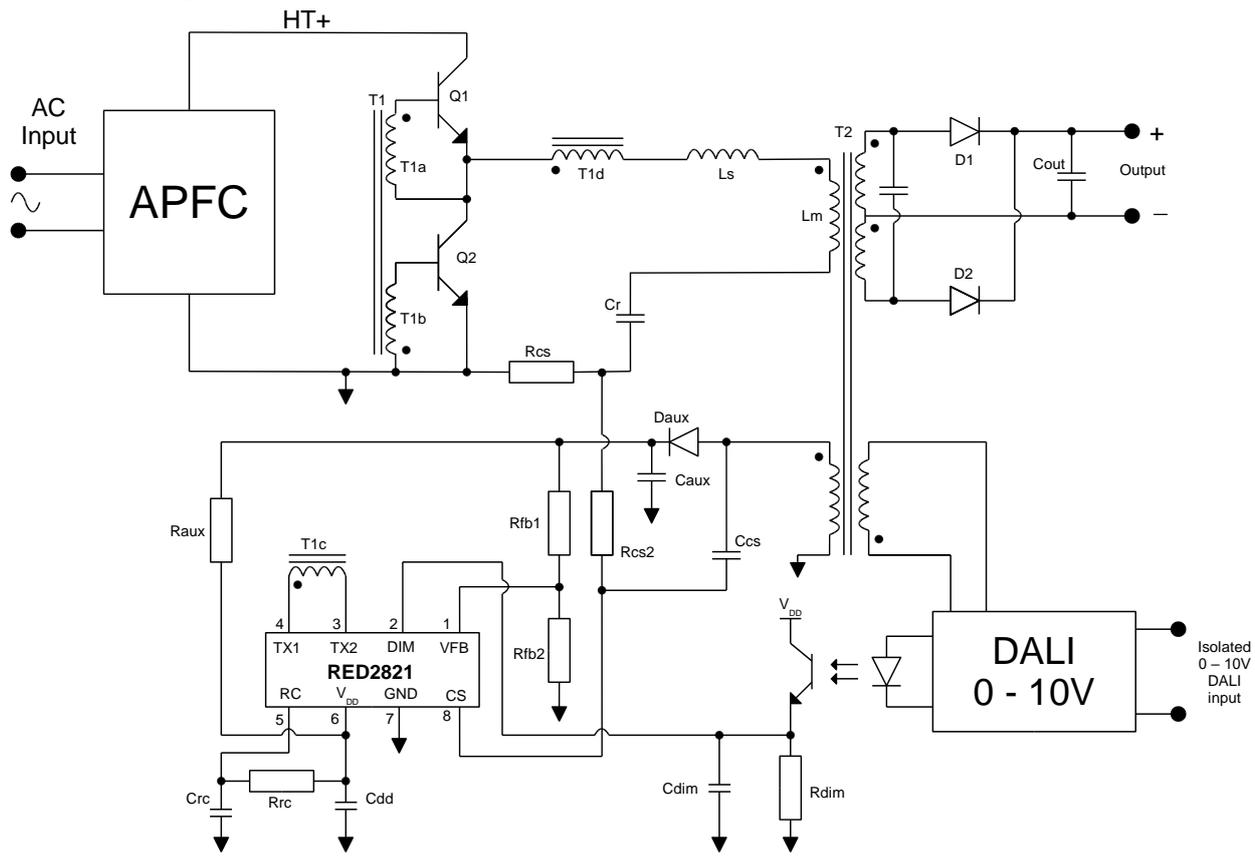
Figure 3: Typical Application : 2-stage LED driver with RED2821 LCC PSR controller and isolated DALI / 0-10V dimming input
