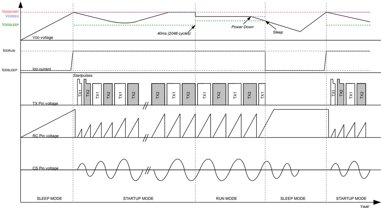
Figure 5: IC Start-up waveforms
