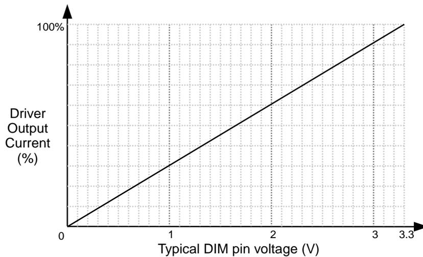
Figure 9: DIM pin voltage vs output current
