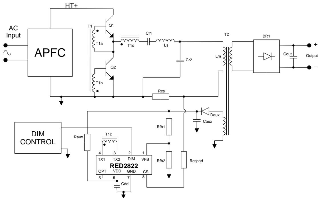
Figure 3: Typical Application: LED driver using RED2822 LCC controller
