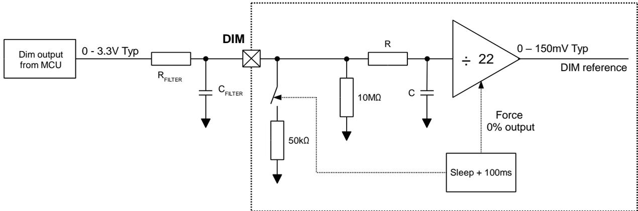
Figure 8: RED2822 DIM pin circuit
