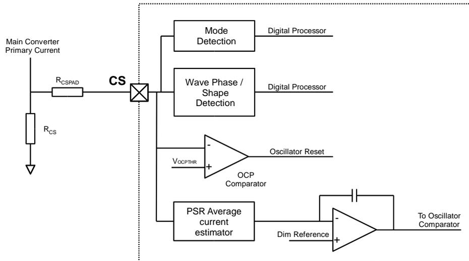
Figure 7: CS Pin connection
