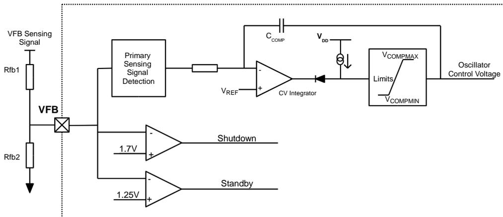
Figure 6: Voltage Error Amplifier Circuit
